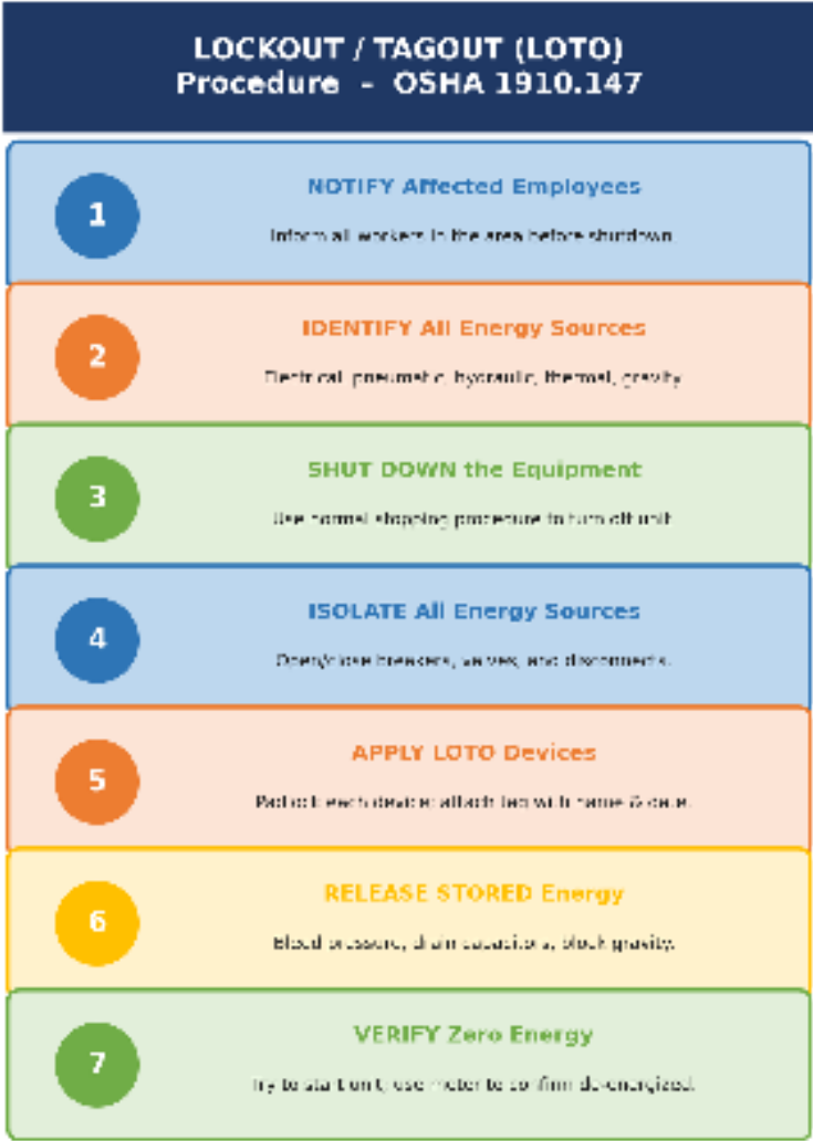
Figure 12-1: LOTO Seven-Step Procedure (OSHA 29 CFR 1910.147)
