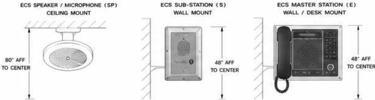
6. TYPICAL DEVICE MOUNTING DETAILS
