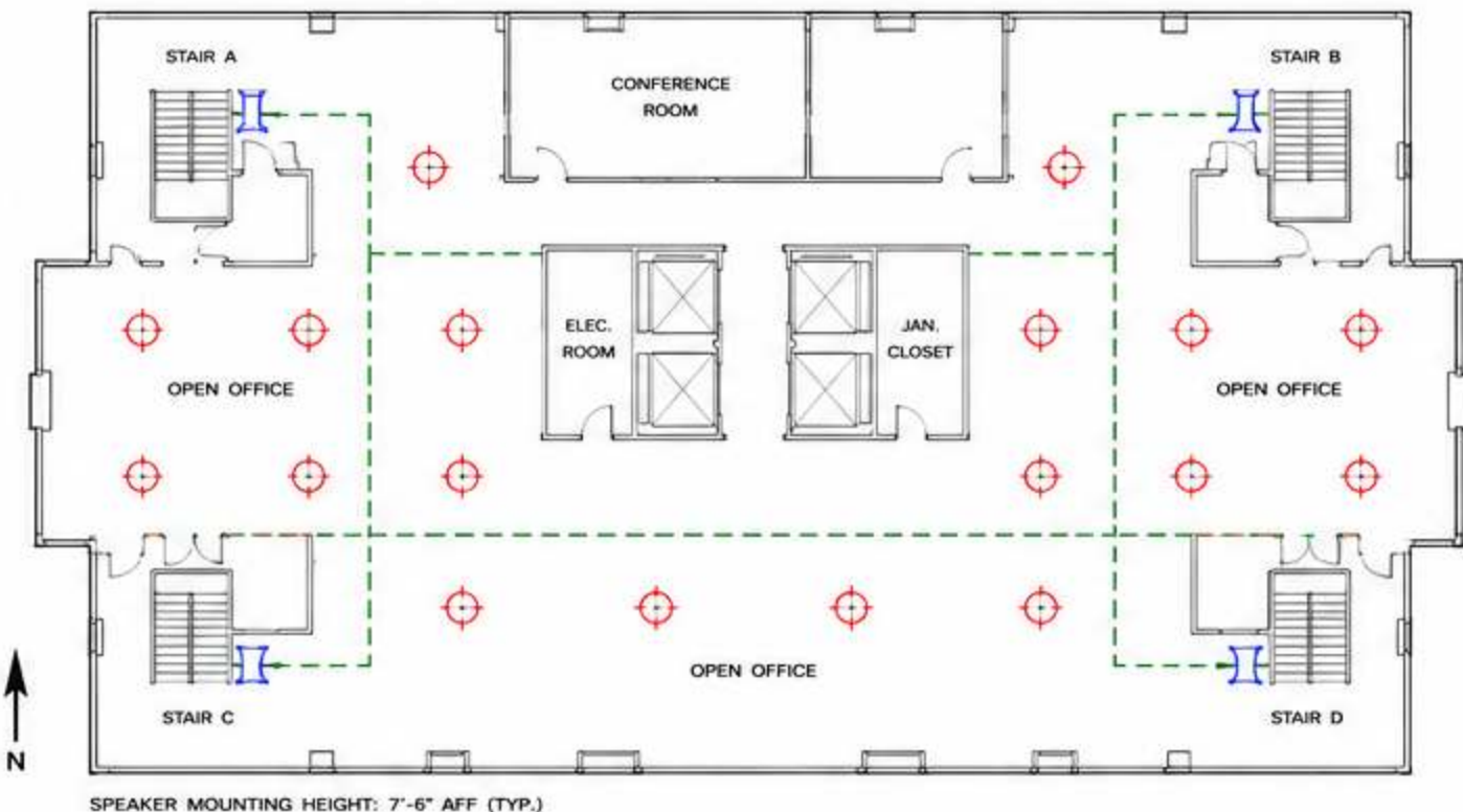
5. SPEAKER WIRING DIAGRAM (CLASS B)
